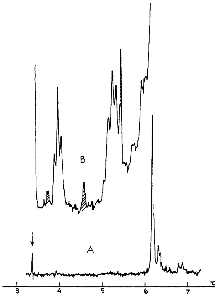
FIG. 1. NMR spectra of (vinyl chloride-vinylidene chloride) copolymer with 90% vinylidene chloride. Solvent, hexachloroacetone. T^{\circ}\text{C} = 130 . A: Single scan spectrum. B: Accumulated spectrum (256 scans). The arrow and the cross-hatched spectra indicate solvent impurities).
